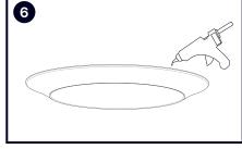
6. The edge of the fixture and the ceiling use waterproof silicone to seal.
