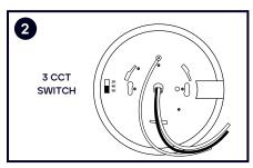
2. Select Color Temperature on CCT Switch located on the back of the fixture.
