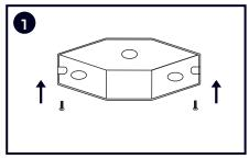
1. PRIOR TO INSTALLATION. Please install two screws (furnished) into the junction box. DO NOT drive screws completely to the end of the junction box.
