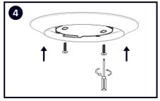
4. With a Phillips screwdriver, attach the disk light lightly to the j-box.
