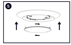
5. Complete the installation by twisting the diffuser on the disk light aluminum enclosure and lock the diffuser in place.
