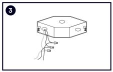
3. Connect supply wires to wires in fixture wiring box with proper size wire nuts or push wires into "push-in" connector. Connect white to white, black to black, and green or bare copper to bare copper wire. The ground wire at the service junction box may need to be secured to a ground screw.
