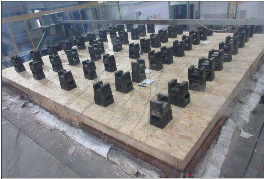
The eunxposed face after test duration of 120 minutes
