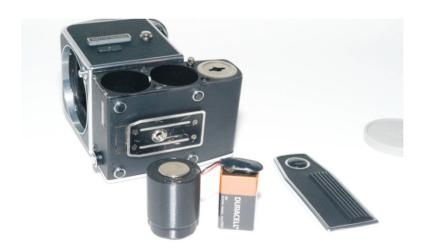
Battery not included with adapter. Compatible with Hasselblad 500EL, 500EL/M and 500ELX. Adapter and battery are inserted in orientation as per picture. There will be slight buckling in the battery cover due to cable connecting adapter and battery. This is normal for 9V adapters
