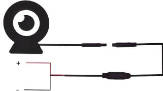
**Step 1:** Locate the drum anchor winch wiring on your boat. Connect the red wire of the power cable to the positive and black wire to the ground. Turn on the camera to estimate the best area you'd like to install the camera. Mark or otherwise take note of the desired location for installation.
