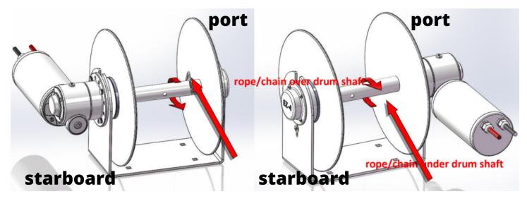
For example - Installing the Rebel winch with the gearbox and motor on the port side will require the rope to
