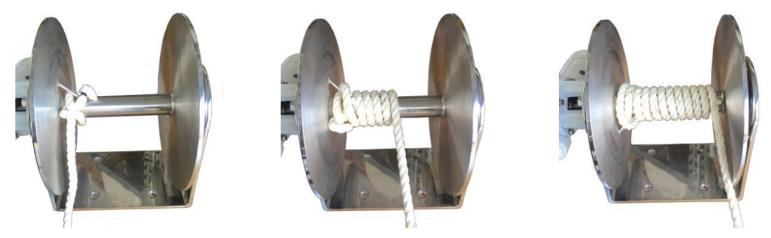
EZ-1, EZ-2 or EZ-3 then either tie it back onto itself or attach with a shackle and wind the rope onto the drum.
