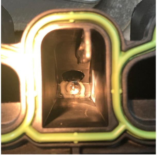
7. At this point, the epoxy should have bonded to the screw, the washer, the surface of the port, and should have been pressed through the outer holes on the port to produce an excellent bond. Note: do not block off the port coming up out of the manifold that the corrugated hose connects to!
