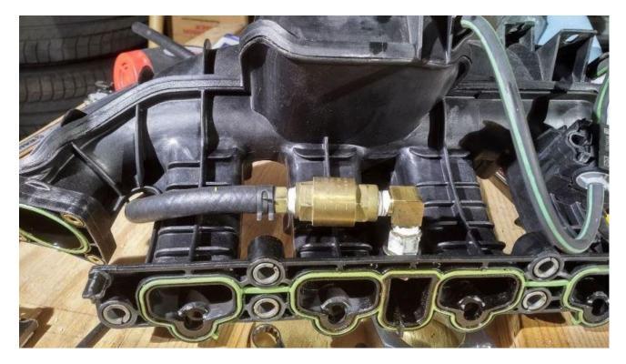
13. Attach the Y fitting to the EVAP purge line. Method 1 is to attach the Y fitting directly to the EVAP purge valve line. To do this, cut the EVAP purge valve line 2-1/4" away from the terminal, then trim 5/8" off of the other end (the check valve side). Hold the Y fitting in a vice, spray it with silicone spray, and slowly heat the nylon line while pressing down on the line firmly.
