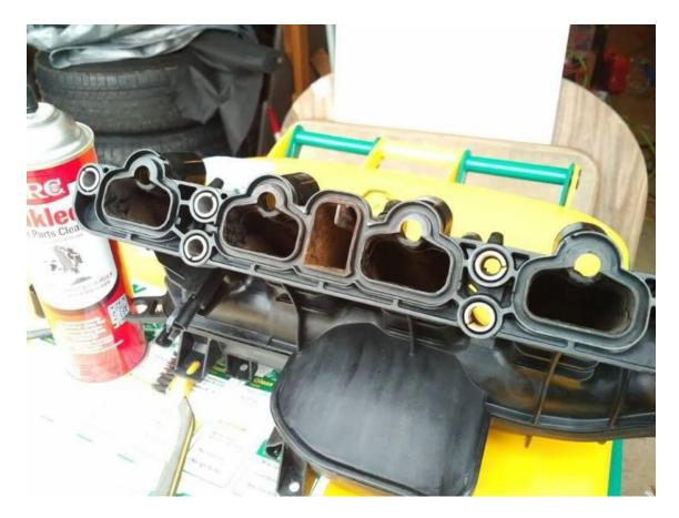
3. Below is where you will be installing the screw and washer. The idea is that if your check valve is missing that hole needs to be plugged up as it's creating a boost leak. First, drive the screw half way into the center hole for the check valve dry (without any epoxy) to start the thread, then back out.
