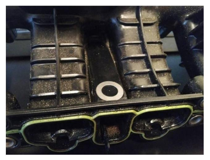
6. Using a step bit, slowly and carefully drill down to 9/16", being sure to keep it centered. If you have trouble getting it centered, you can try drilling a small 1/8" pilot hole with another drill bit first. Note that the hole on mine ended up a little too close to the opening. This is why I recommended you start further back to give you some flexibility in case this happens.
