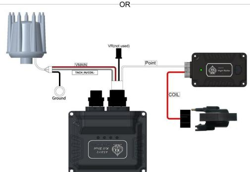
The loose wire "Point" provides an ignition signal from the KILLSHOT™ ECU to another module like the ACES HIGH ROLLER™ CDI box.
