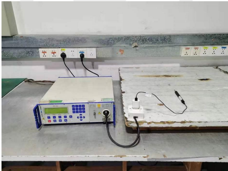
15.6.Photo of Electrical Fast Transient / Burst Test
