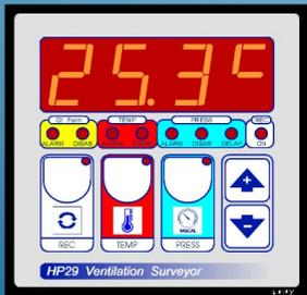
Independent ventilation alarm unit which is a supplementary source of the following alarm:
