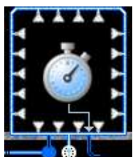
The air valve is open and the drain valve closed for the delay time
