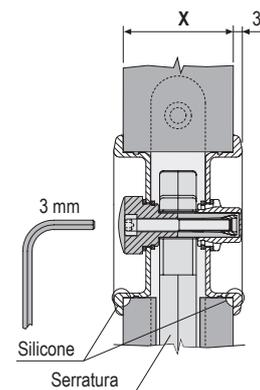
ANELLO COMPENSATORE  $\varnothing 48$  MM DA ABBINARE ALLE MANIGLIETTE B01920.02. XX PER CAMPI DI APPLICAZIONE 36+40 MM
