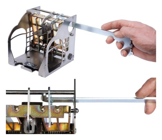
2. Once the trap is positioned in the tunnel, hook the safety catch through the round hole in the side of the trap and remove safety as described in the main trap instructions.
