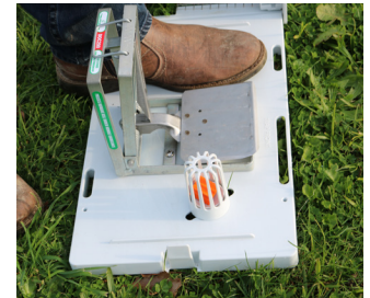
4. Make sure the bottom of the Waddington trigger is resting on the front face of the pierced tab on the treadle plate.
