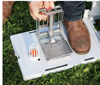
2. Place foot on base of housing, lift trap kill bar to set position over Waddington trigger. The Waddington trigger will fall towards the treadle plate.
