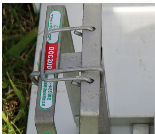
5. Lift kill bar and secure safety clip as shown and proceed to remove dead pest.
