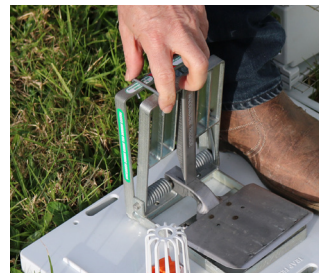
6. Once clean, remove safety clip while maintaining hand pressure on the kill bar. For re-setting follow steps 2 - 4.
