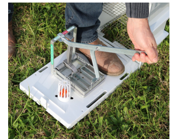
When using the Doc Setting Tool place tool to the right hand side of the Waddington trigger. For re-setting follow steps 2 - 4.
