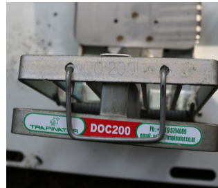
3. Carefully lower the kill bar to engage the top edge of the Waddington trigger.
