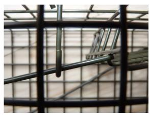
Step 5 When set, the treadle plate should be raised from the base of the trap.
