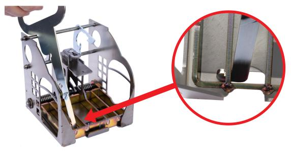
1. Place the hook of the setting tool through the gap in the end of the 2nd bar.
