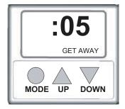
TEST FEEDER: PRESS AND HOLD the SET button while the RUN-TIME SECONDS are displayed. Release the button and get away from the feeder when the message "TESTING GET AWAY" appears on the display.
