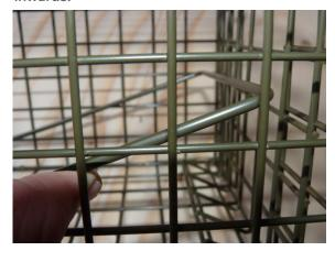
Step 3 Place rod under first bar of door. Ensure rod is resting inside wire cradle.
