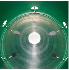
2. Then place the cone into the feeder, making sure it sits flush with the base and is not resting on any bolt heads.
