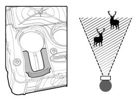
Push the Zone Control shutter down for wide detection.
