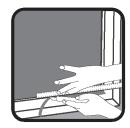
**A.** To trim the excess film, firmly press down on the edge of the window using cutting stick and trim excess film with trimming knife. Repeat step 2B to finish installation and ensure all solution is removed from under the film.
