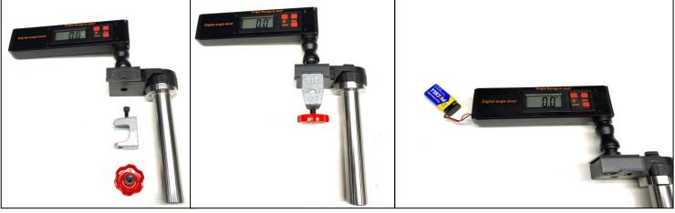
Note: (Do not rotate the drive pin more than -15° counterclockwise or 240° clockwise. Also, do not swing the display head more than a couple turns in the same direction, as you will rip the power cord you just soldered.)
