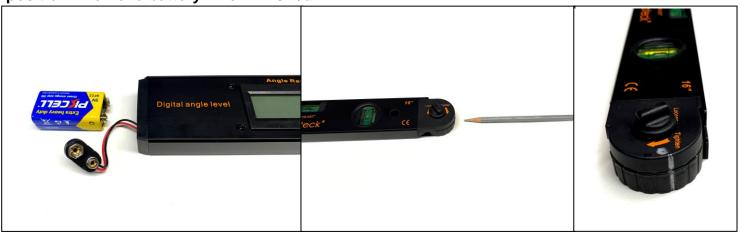
Step 3: Remove the aluminum back plate and mark cut locations.
