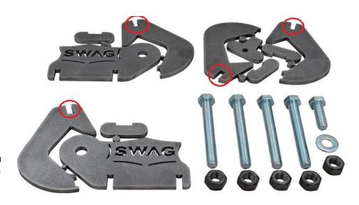
Separate all the steel plates by breaking them apart, then welding up the kit as shown below. When welding on the  $(4) \frac{1}{2}$ " weld nuts make sure that the nuts line up with center of the large "V" cut outs.
