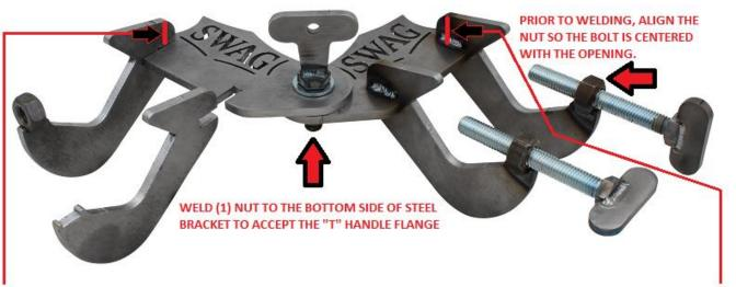
THE HEIGHT OF THE LEFT "J" HOOK BRACKETS ARE A SHORTER DISTANCE THAN THE "J" HOOK BRACKETS ON THE RIGHT SIDE
