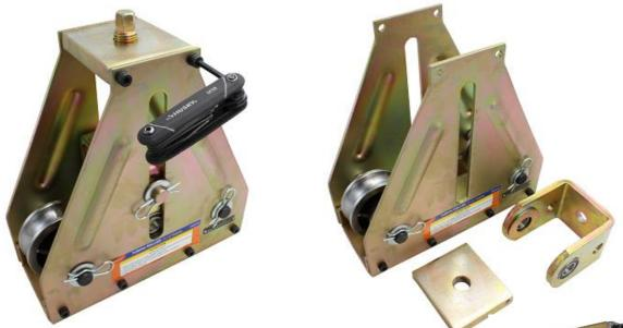
**Step 3.** Install the (2) side plate extensions and spring retainer plate as shown below, using the provided (4) 5/16" bolts and lock nuts on the bottom, The (4) metric fasteners that were previously remove will be reinstalled on top threaded plate.
