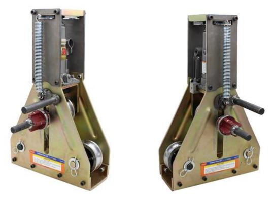
**Step 9.** Finished assembly. Note you will need to add grease between bottom spring mounts and the tubing roller frame to ensure the assembly slides freely up and down.
