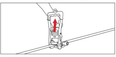
While holding the release lever in horizontal line, pull the ratchet all the way open until it is released, then pull the line out from the straightened end.
