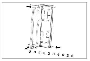
6. Place the glass according to the schedule and fix it withe the nuts.
