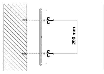
1. Fix the crossbar to the wall by using wall mounting plugs and screws suitable to your wall type.
