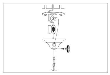
3. Hang the lantern on the hook of the ceiling plate with the canopy at the lowest position. Carefully lower the lamp until the chains is taut. Straighten the chain links.
