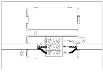
2. Connect the 3 wires according to their colours. Brown is the live wire (L), blue is the neutral wire (N), green/yellow is the earth wire ( $\frac{1}{-}$ ).
