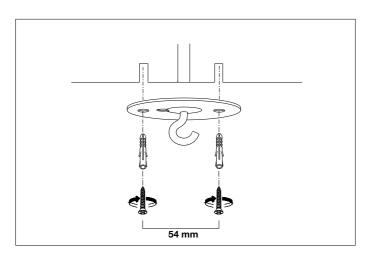
Fix the ceiling plate to the ceiling by using mounting plugs and screws suitable to your ceiling type. Make sure to lead the wire through the plate.
