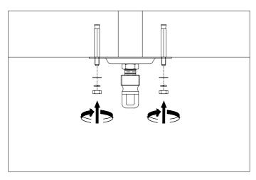
Lead the wires from your ceiling through the hole of the ceiling plate. Fix the ceiling plate to the ceiling by using mounting plugs and screws suitable to your ceiling type.
