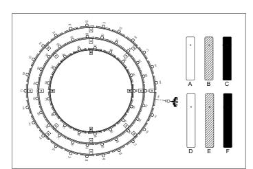
5. Place the glass according to the schedule from the inner ring outwards. A, D is clear glass, B, E is light smoke glass and D, F is dark smoke glass.
