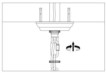
3. Slide the canopy over the ceiling plate. Hang the lamp from the suspension eye, using the chain and carabiner. Carefully lower the lamp until the chain is taunt. Straighten the chain links.
