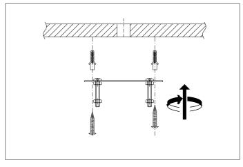
2. Lead the wires from your ceiling through the hole of the ceiling plate. Fix the ceiling plate to the ceiling by using mounting plugs and screws suitable to your ceiling type.
