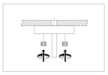
**4.** Place the ceiling canopy over the ceiling plate and fix it securely with the nuts.
