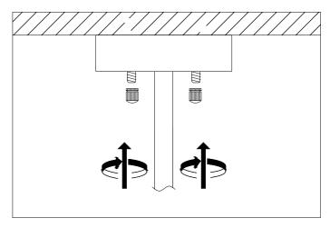
$\textbf{4.} \ \textbf{Place the ceiling canopy over the ceiling plate and fix it securely with the nuts.}$
