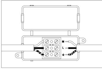
3. Connect the 3 wires according to their colours. Brown is the live wire, blue is the neutral wire and green/yellow is the earth wire.
