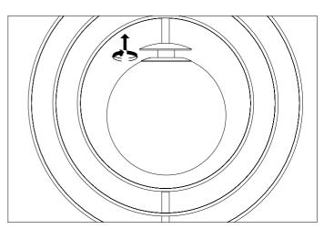
**6.** Place the alabaster glass and adjust the rings to the desired position.
