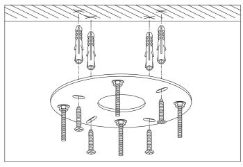
2. Fix the ceiling plate to the ceiling by using mounting plugs and screws suitable to your ceiling
