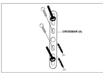
1. Fix the cross bar to the wall by using wall mounting plugs and screws suitable for your wall type.
