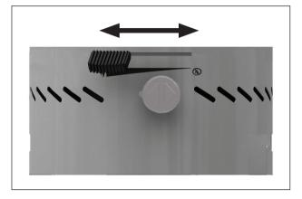
With your heat-resistant ash container handy, remove the ash catcher from its position and carefully dump all ashes into a heat-resistant container. Allow it to sit for 24 hours.
