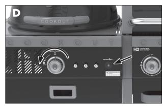
8. After charcoal has ignited (approximately 5 minutes), press in and turn the gas ignition burner to the OFF position.
