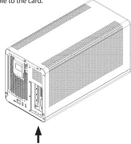
4) Reinstall the sliding cover and screws.
