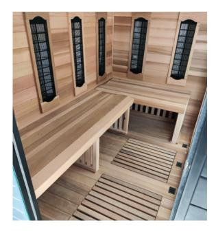
16. Next install the backrests. Place the backrests against the wall and the sides aligned with the holes in the wall. Connect wire from the top of the backrests to the wire that comes through the wall for the LED lights. Use the screws for the backrest to attach the backrest to the wall using the pre-drilled holes in the backrests.
