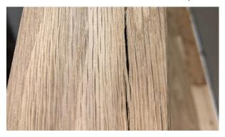
End-Checks - Like surface checks, end checks occur in, or adjacent to, the wood rays, but on the ends of the boards rather than the face. These separations occur due to the normal movement of moisture along the length of the boards, where the ends of the boards dry more rapidly leading to stress fractures on the ends of the boards.
