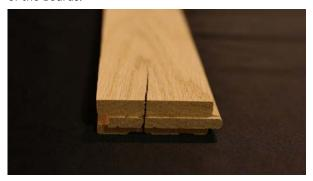
Internal Checks (Honeycomb) - An internal defect in the wood that may not be visible on the surface of the board, but occurs in the core (inner part of the board) of solid boards. These checks can become exposed when the boards are sanded or milled. They can also become exposed on the surface of the board with a loss in moisture or changes in RH after installation.
