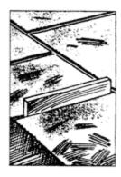
4. Maintain a grout space between the pieces as recommended by the slate supplier (1/4" or 3/8") depending on the size of the tiles. To do these accurately, use spacers.
