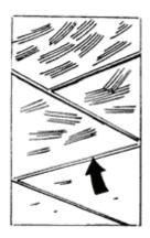
2. Add water slowly while mixing to get the texture of damp sand mix grout according to the manufacturer specs, and apply with a grout float to press grout deeply between the joints. Mix only enough grout to be used in about 30 minutes or difficulty will result in hardening in the pail.
