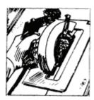
7. Slate tile can be easily cut with a wet saw using a diamond blade
