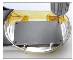
Please note: do not align the template bracket to the flat top side of the frame, this section is not level to the ground. The
