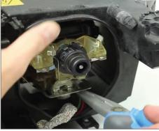
Unclip the top hinge. Remove the frame from the housing. Rotate it further downwards and slide it over the ball hinge. Remove the projector bowl by removing all the Torx screws. Unclip and remove the shroud and lens frame. Also remove the rubber rings inside the mounting holes don't throw them away!
