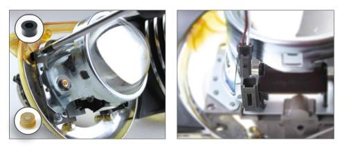
Plug-in the solenoid cables into the female connector at the front of the projector. Make sure the solenoid cable is quided to the back of the reflector.
