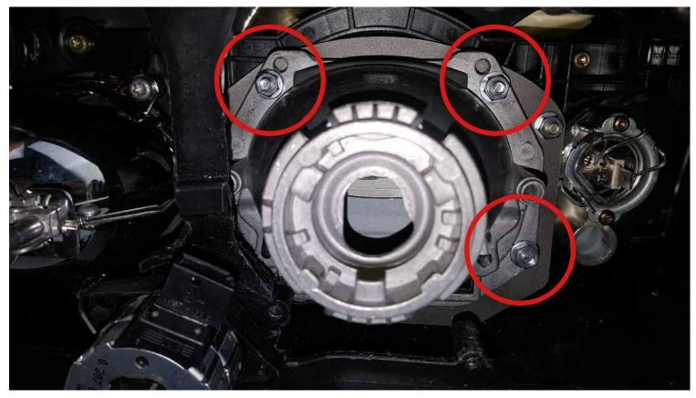
Put the projector in position and push the projector on the exposed threads. This can also be a bit tight and some (delicate) force may be needed to push the projector on the threads. After this add the rings and nuts and fasten the nuts.
