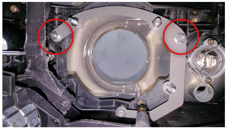
Add the rings and nuts to the top 2 mounting points and fasten the nuts. The bracket is now secured to the original mounting points.
