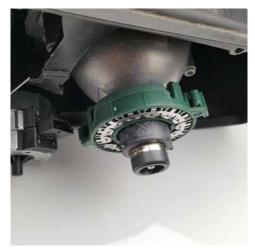
Twist the bulb and ring on to the projector.
