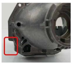
A little piece of material needs to be removed from the new Aharon Optimus NT projector to clear the height adjustment assembly. This can be done with an angle grinder, hack saw or Dremel for example.
