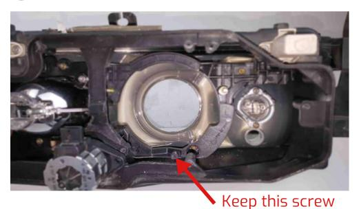
Remove the original projector and hardware from the threads. (and feel how light the plastic projector is).
