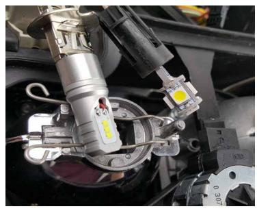
Optionally connect and mount the H3 LED bulb for the fog light and/or the T10 LED for the position light.
