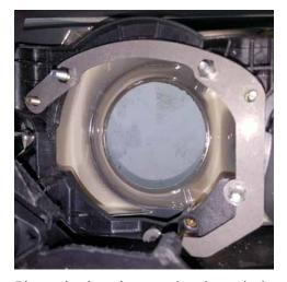
Place the bracket on the threaded mounting points (can be a bit tight).
