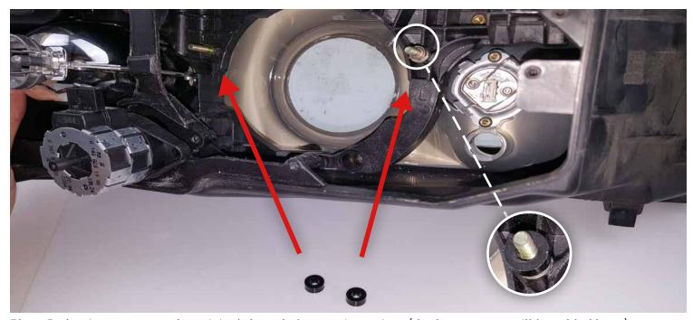
Place 2 plastic spacers on the original threaded mounting points (the bottom one will be added later).
