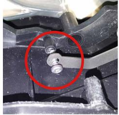
Now place the bottom screw thought the bracket.
