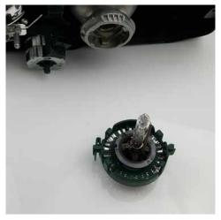
Close the ring with the guiding pin positioned in the notch in the bulb.
