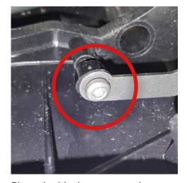
Place the black spacer on the screw and direct the screw to the hole and fasten the screw.
