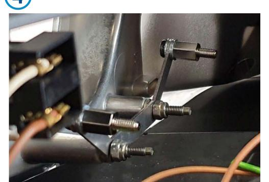
Mount the bracket onto the threaded mounting points, positioned at the bottom of the headlight. Use the M4 lock nuts, that were used to mount the OEM projector, to secure the bracket.
