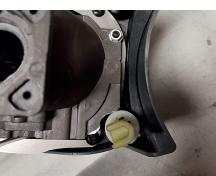
A small piece of the projector needs to be trimmed for the plastic holder/retainer, try to align it with the bracket.
