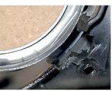
Trim a piece on the inside of the headlight to make sure the solenoid of the projector will fit.
