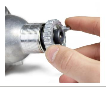
To secure the bulb you need to clamp the bulb with the provided metal spring and the metal nut, this can require a bit of force.
