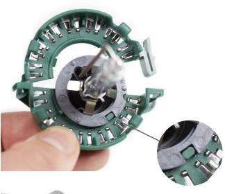
Open the green bulbholder and insert the lamp into the bulbholder. Be sure to allign the lamp and the holder as shown on the picture. After being properly alligned, close the bulbholder again.
