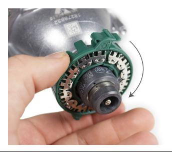
Now simply turn the bulbholder clockwise to secure the lamp into the projector.
