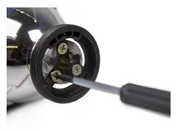
1) Install the bulb holder with the 3 screws supplied. The holder only fits 1 way.
