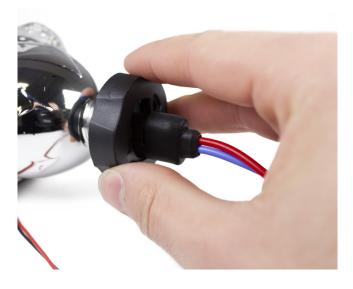
H) Now simply slide the plastic nut towards the shaft and turn it clockwise to secure it.
