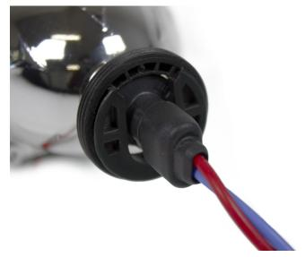
3) To secure the lamp in position you need to place the plastic piece as shown above.
