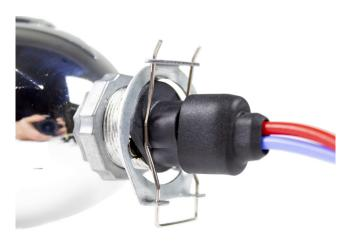
4) Now with a bit of force, push the spring under the hooks of the mounting plate.
