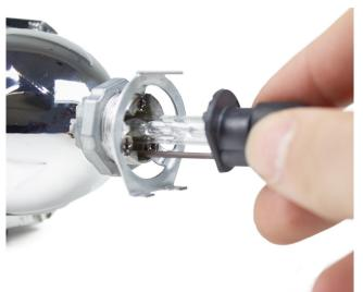
Insert the lamp into the shaft, do this carefully not to damage the lamp.
