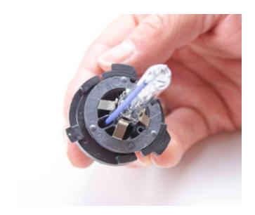
Mount the bulb holder parts onto the D2S xenon bulb, like shown in the pictures.
