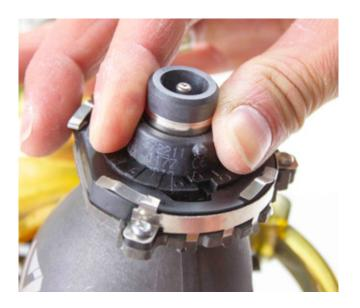
Insert the bulb into the shaft of the projector (with the bulb tube facing down) and twist the bulb clockwise until the little pins on the bulb align horizontally.
