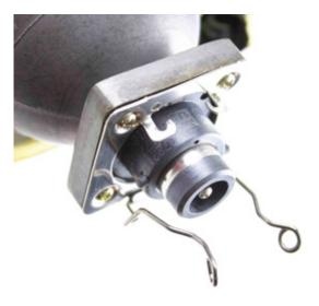
Insert the bulb into the shaft of the projector (with the bulb tube facing down).
