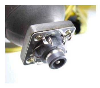
Tighten the clip and check if the lamp is securely in place.
