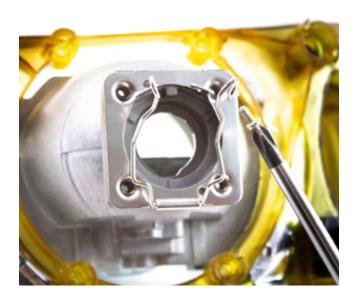
Mount the bulb holder onto the back of the projector using the 4 supplied screws. Make sure the pivot point is facing the bottom of the projector.
