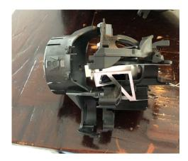
It is quite hard to remove the projector through the back of the headlight but possible ... If needed, the projector can be dismantled a bit and can be removed in parts.
