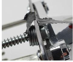
In order to mount the bracket inside the headlight you need to use the supplied M4 rings (4 per side) and the original Torx screws. Easiest method is to retain the rings with a little piece of tape.
