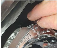
The tape can be removed after the screws are screwed onto the frame of the headlight.
