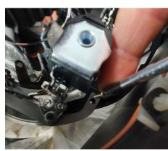
The supplied screw can be used to secure the bracket at the bottom.
