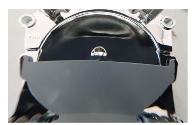
The cut-off plate of the new projectors is a bit too wide to fit the headlight frame. It needs to be trimmed about 3 mm per side.
