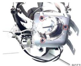
Mount the D1S bulb holder onto the Aharon E46-r projector using the small 3 screws supplied with the holder.
