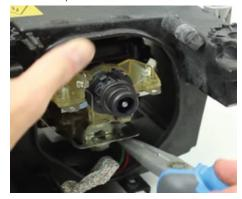
Unclip the top hinge. Remove the frame from the housing. Rotate it further downwards and slide it over the ball hinge Remove the projector bowl by removing all the Torx screws. Unclip and remove the shroud and lens frame. Also remove the rubber rings inside the mounting holes.
