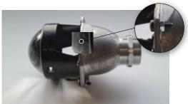
Mount the projector to the bracket using the washers and nuts.
