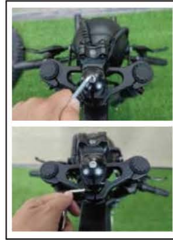
8.Install retainer and top cover and tighten all screws
