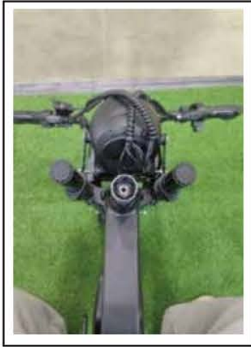
7.Put the steering in front
