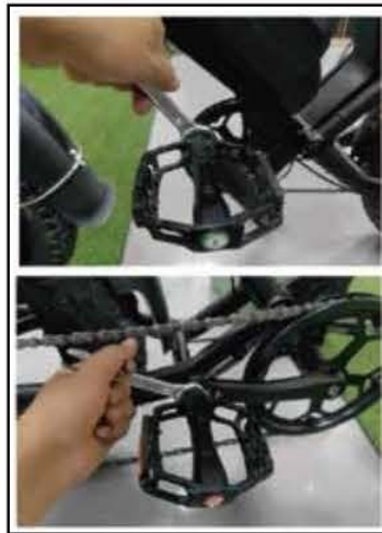
16. Install the pedal and tighten the screw
