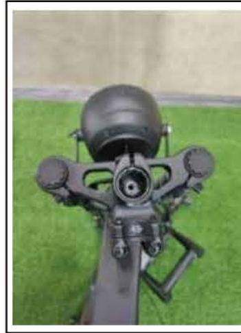
5. Unscrew the screw and remove the trim cover
